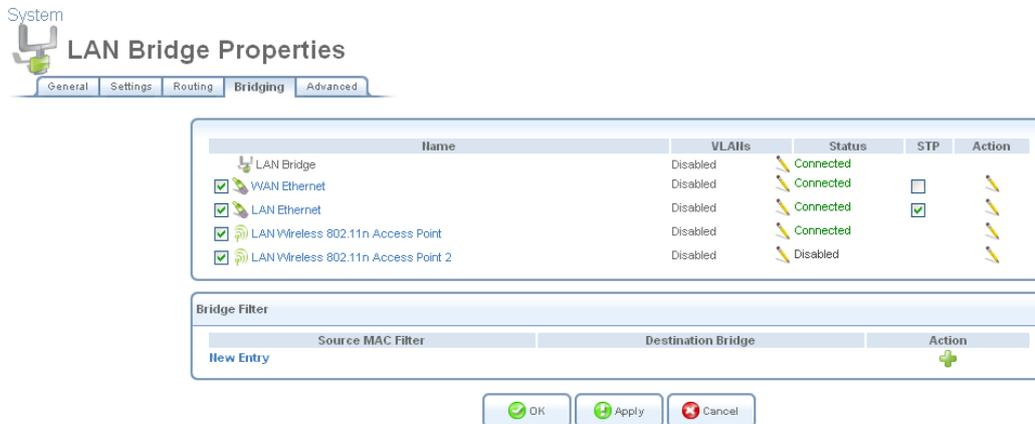
**Figure 6.251 Bridging tab of LAN Bridge Properties**
