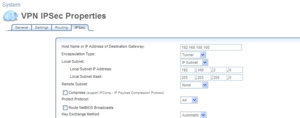
**Figure 5.78 VPN IPsec Properties – IPsec**
