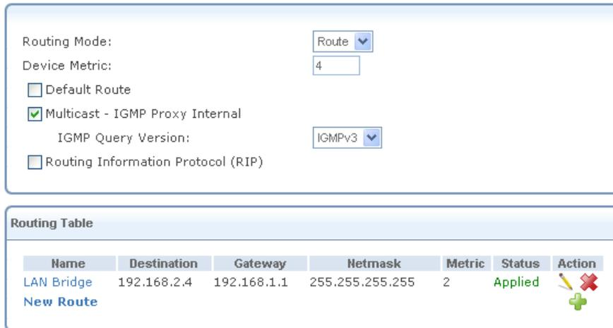
**Figure 6.132 Advanced Routing Properties**
