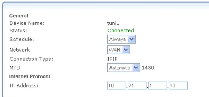
The screenshot shows a configuration window titled "General" for a tunnel named "tun1". The status is "Connected". The "Schedule" is set to "Always". The "Network" is set to "WAN". The "Connection Type" is "IPIP". The "MTU" is set to "Automatic" with a value of 1480. The "Internet Protocol" section shows the "IP Address" as 10.71.1.10.
