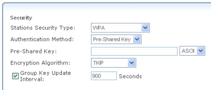
Figure 6.69 WPA Wireless Security Parameters
