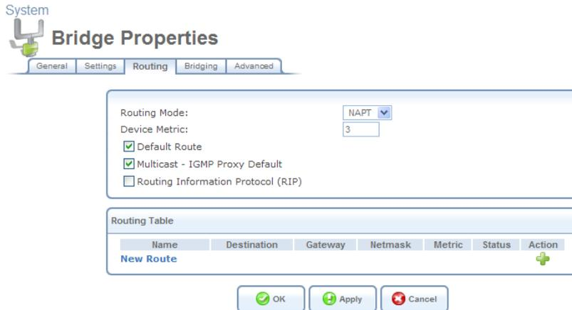
**Figure 6.171 WAN-LAN Bridge Routing Settings**
