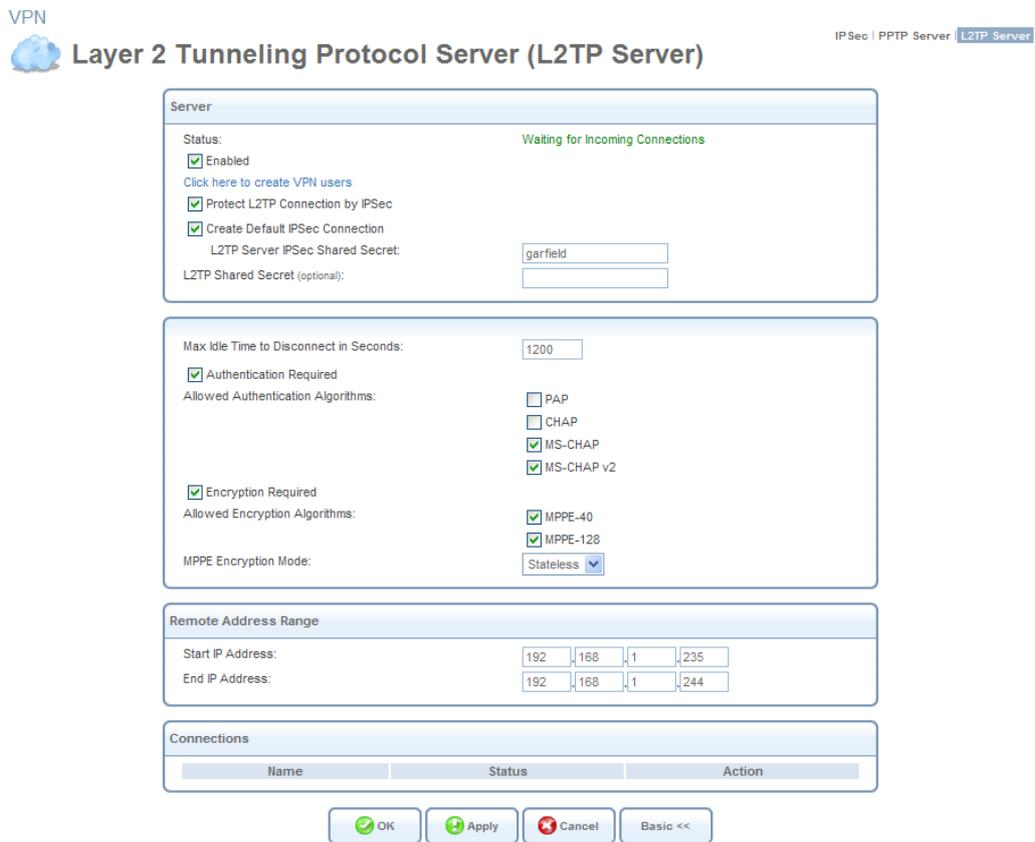
**Figure 6.138 Advanced L2TP Server Parameters**
