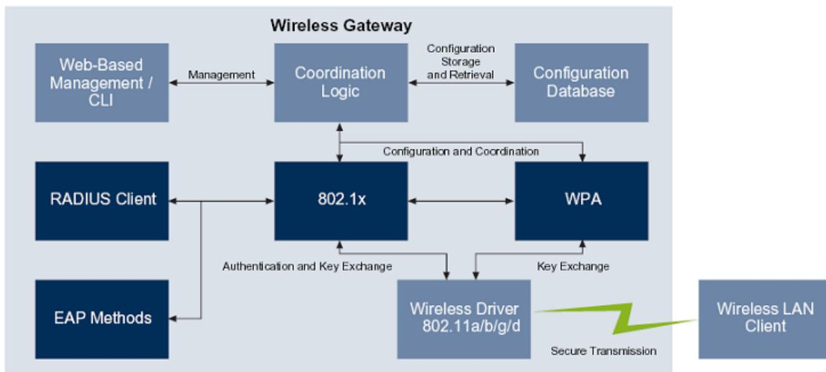
**Figure 6.44 iPECS SBG-1000 for Wireless Gateways – Authentication and Encryption Components**
