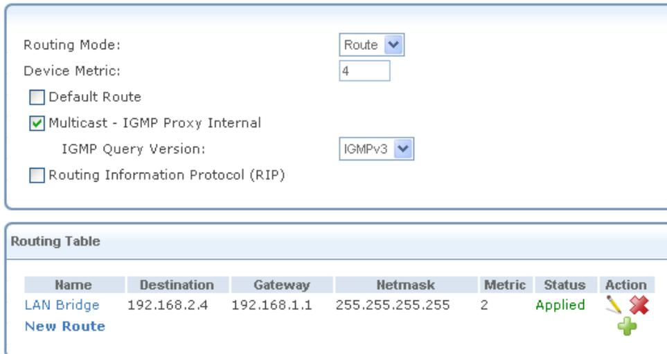
**Figure 6.39 Advanced Routing Properties**
