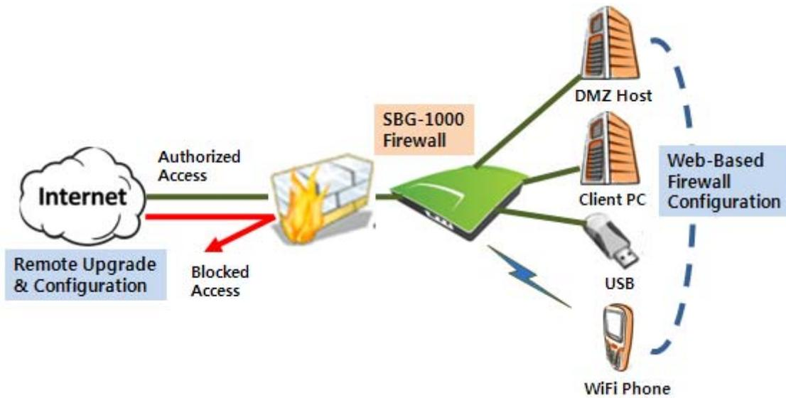
Figure 5.2 iPECS SBG-1000's Firewall in Action
