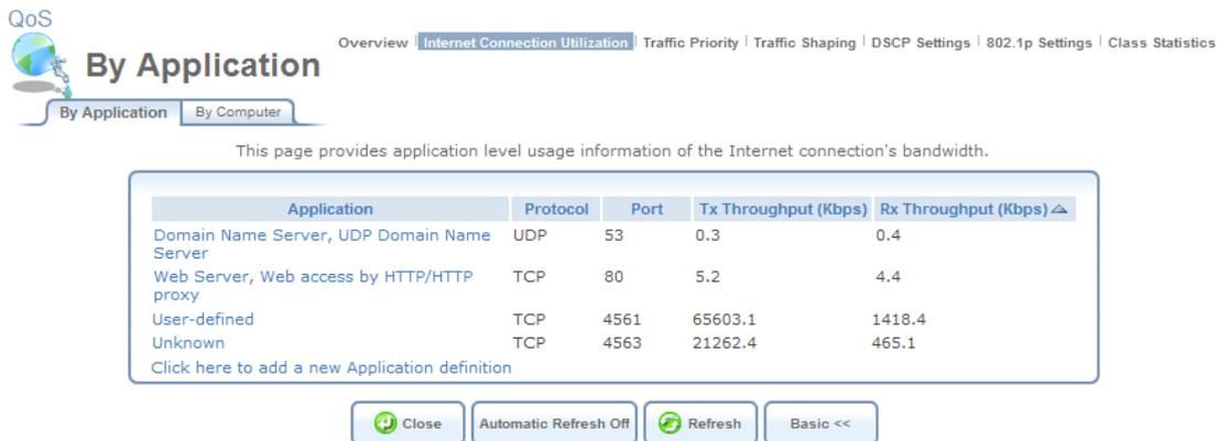
**Figure 5.47 Utilization by Application – Advanced View**
