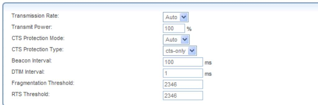
**Figure 6.80 Transmission Properties**
