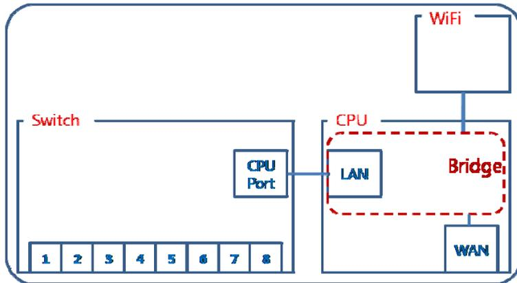
Figure 6.205 iPECS SBG-1000 internal architecture
