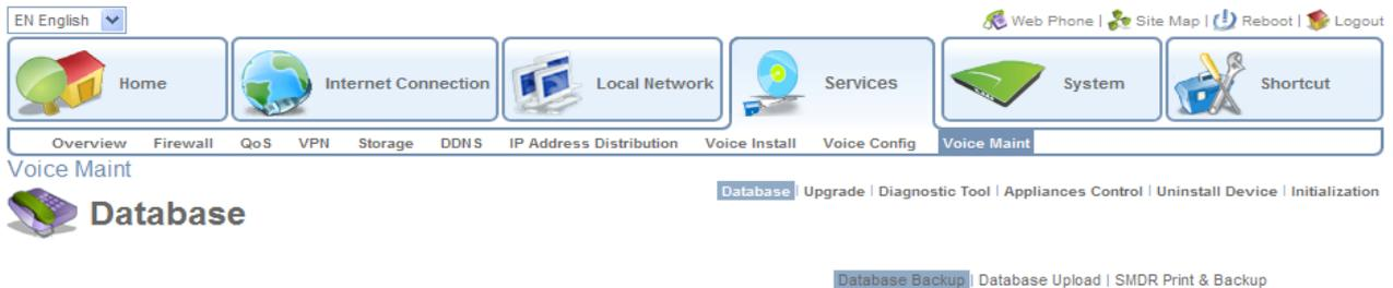
The Maintenance Main menu item permits download of all or portions of the system's database, and downloading and viewing of SMDR data. The user also can set trace direction or target and system logs. Other functions include uninstall registered station, delete voice mail box for each station, and initialize call attributes.
