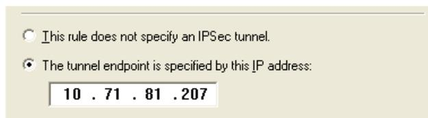
**Figure 5.104 Tunnel Setting**
