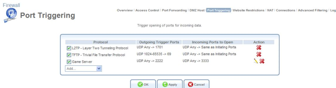
**Figure 5.23 New Port Triggering Rule**
