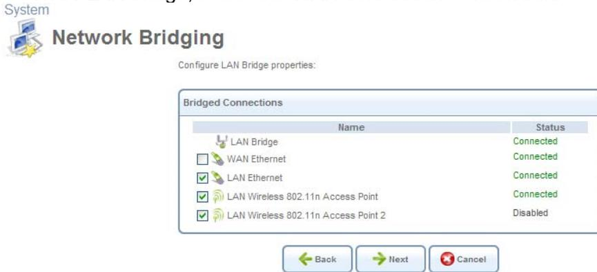
Figure 6.166 Network Bridging – Configure Existing Bridge
