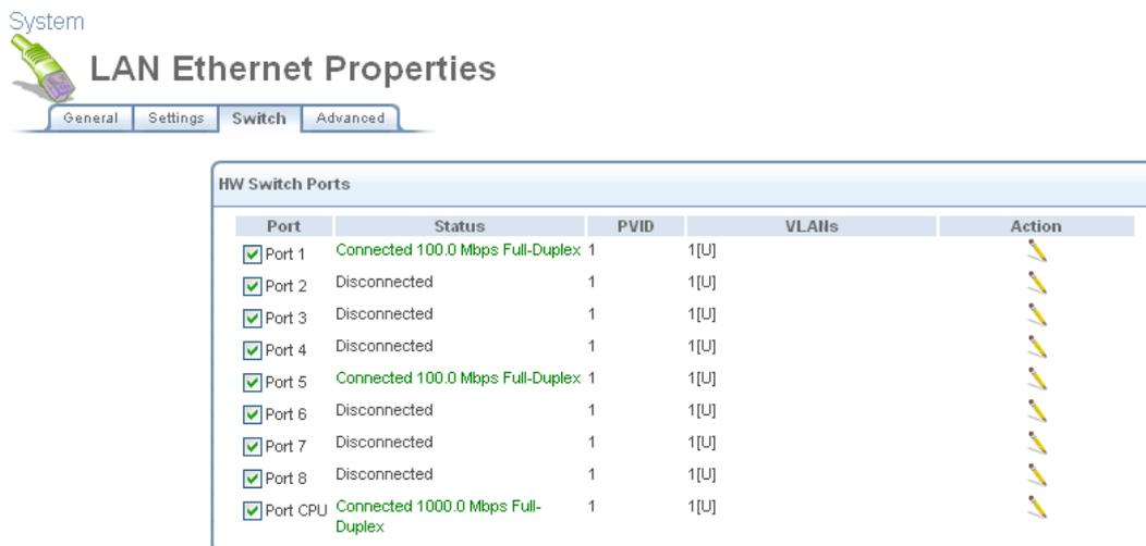
**Figure 6.238 Switch tab of LAN Ethernet Properties**
