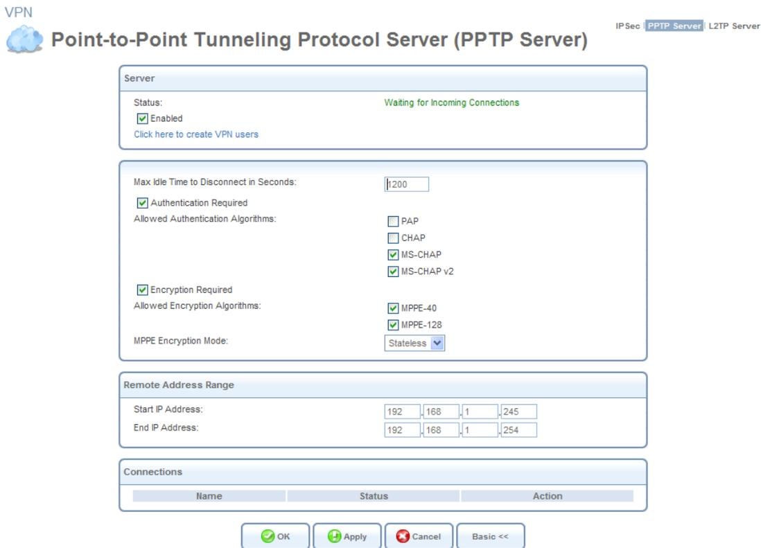
Figure 6.157 Advanced PPTP Server Parameters
