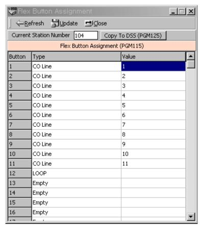
[Figure 4-4] Flex Buttons Assignment Window
