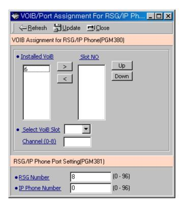
[Figure 13.1] VOIB Slot Assignment for RSG/IP Phone (PGM 380)
