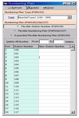
[Figure 3-5] Numbering Plan type Setting Window
