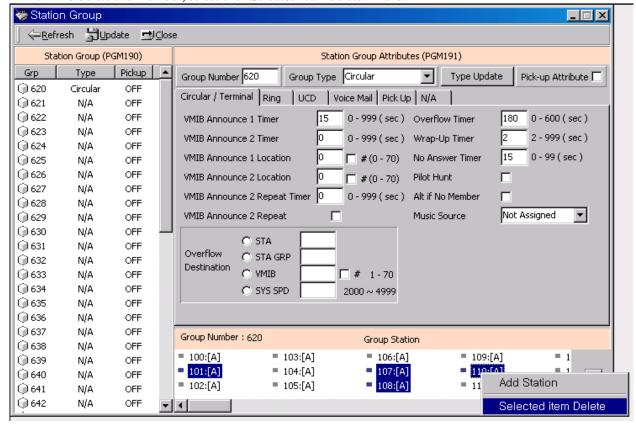
[Figure 7-5] Station member Deletion Assignment
